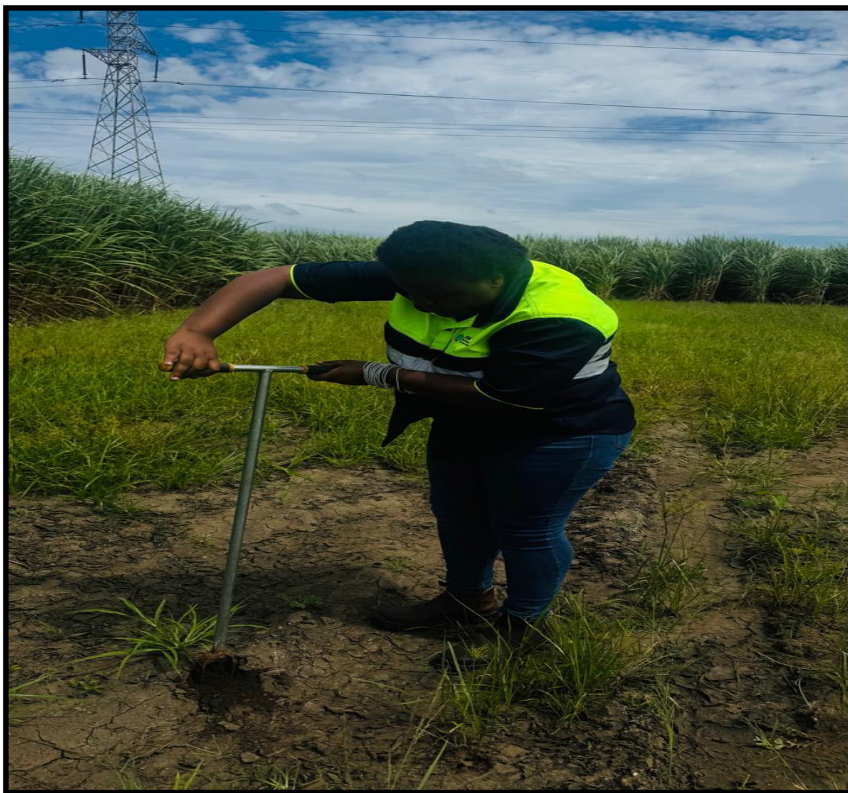
Figure 11 : A field technician collecting a soil sample using a hand auger within a sugarcane cultivation area.
